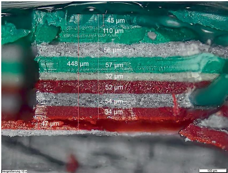
Porsche 356: Image showing cross-section of paint layers under a microscope [20]
