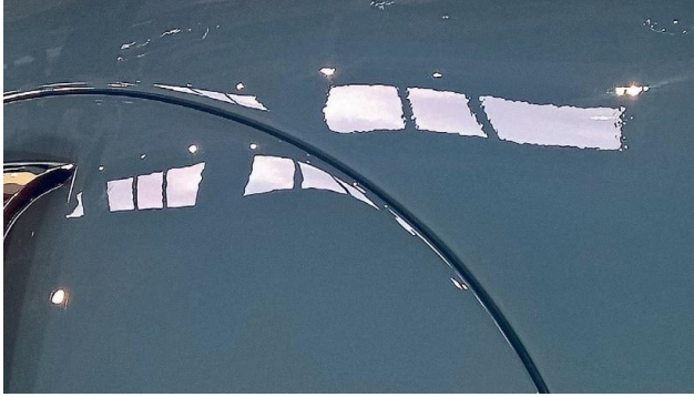
Significant differences in paint flow on the hood and front end of a recently restored Porsche 356
